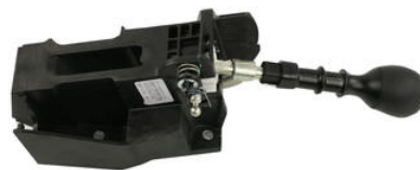
GEAR LEVER MECHANISM IVECO DAILY 06>
